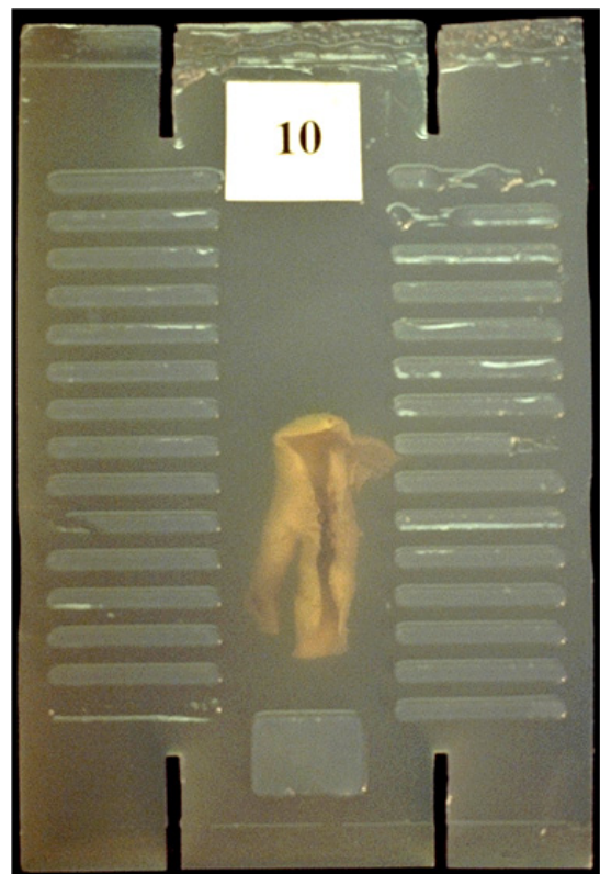
Figure 1 Photo of agar block with atherosclerotic tissue embedded in the agar. The fiducial markers are seen as the two columns at left and right.
