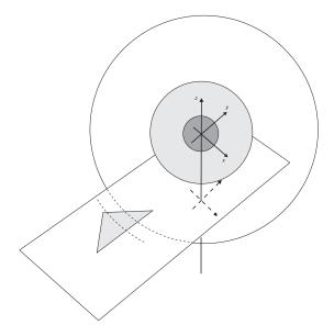
Emission of spherical wave from the field point and its intersection of the aperture.
