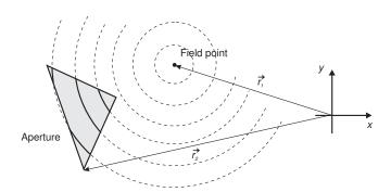
Intersection of spherical waves from the field point by the aperture, when the field point is projected onto the plane of the aperture.
