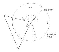
First response arrives at  $t=t_1=z/c$ , hereafter the fixed part of the circle between the angles  $\theta_b$  and  $\theta_c$  contributes to the response.
