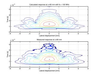
Point spread function for concave, focused transducer
