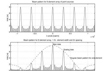
Grating lobes for array with 8 point elements (top) and of 8 elements with a size of  $1.5\lambda$  (bottom). The pitch is  $2\lambda$ .
